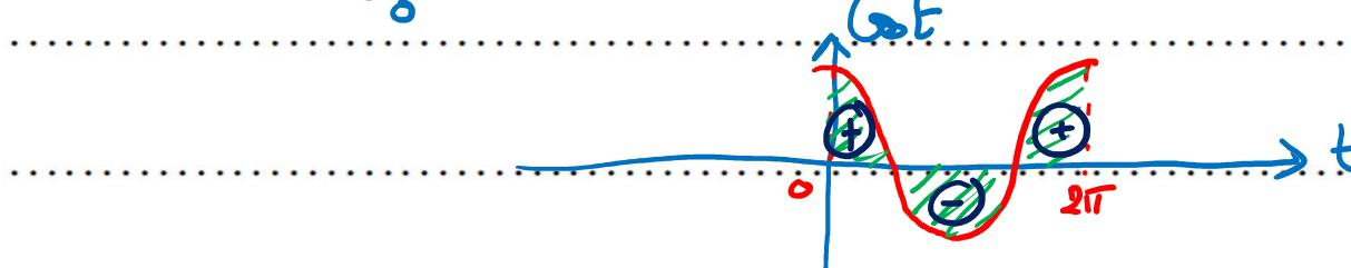
$$V_{\text{eff}} = \sqrt{\frac{1}{T} \int_a^{a+T} f^2(t) dt} \quad u(t) = \cos t \quad T = 2\pi$$
